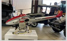
helicopter which they use for highly-targeted application of pesticides in the vineyards. The R-Max is much more efficient than traditional crop dusting using fixed winged aircraft, or even manual application from the ground, especially in steep terrain. Just one example of technology helping to improve one of the oldest activities in human endeavour: winemaking.
